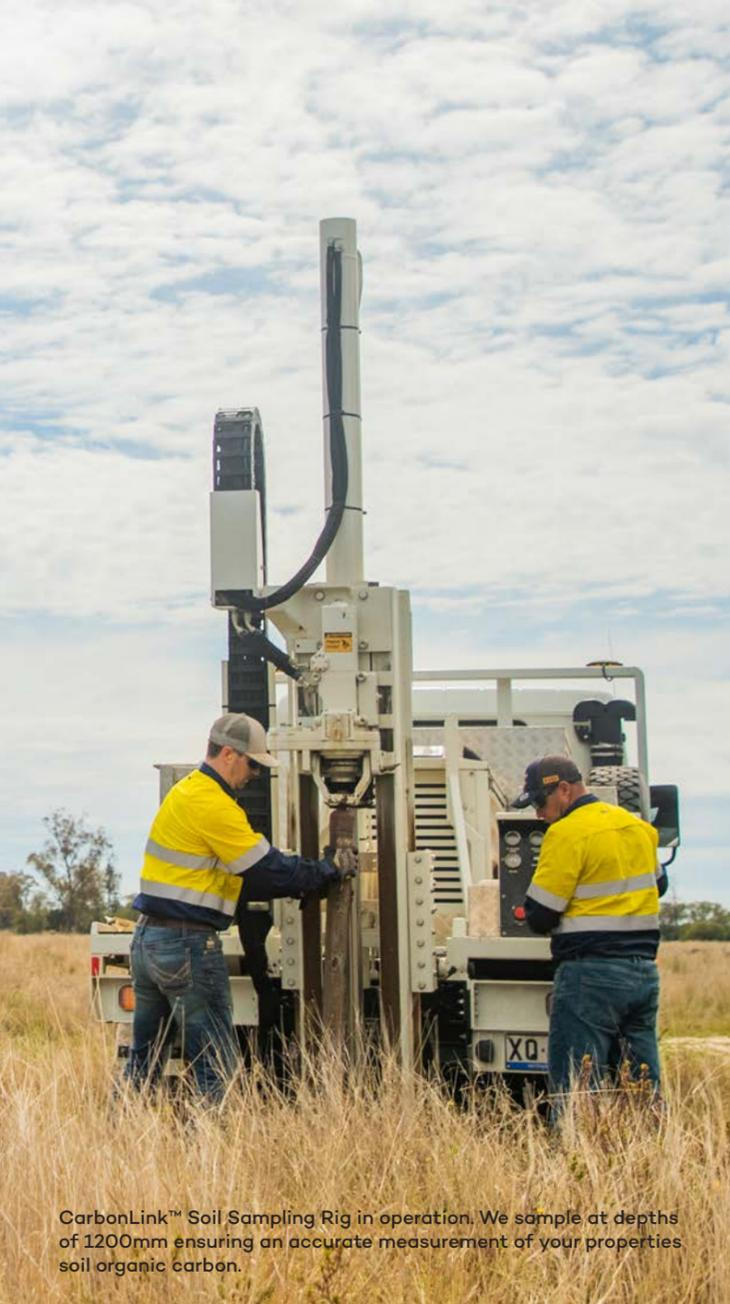
CarbonLink™ Soil Sampling Rig in operation. We sample at depths of 1200mm ensuring an accurate measurement of your properties soil organic carbon.
